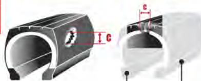
Non repairable area
